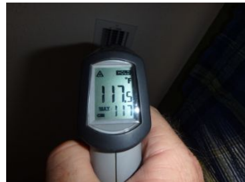
Supply vent heat temp upstairs
