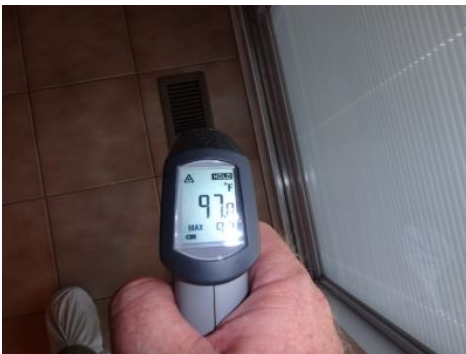
Supply vent heat temp main floor (short run)
