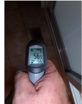
Supply vent cooling temp main floor
