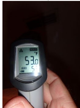
Supply vent cooling temp upstairs
